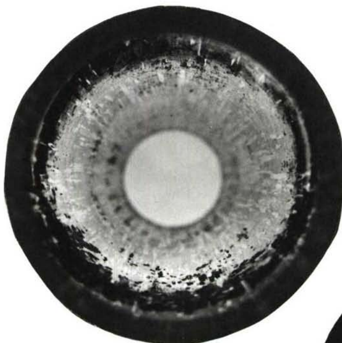
FIG. 8. Barrel L/521. R.A.R.D.E trial, fired 184 bombs obturated with Polycarbonate rings. Breech end view.
