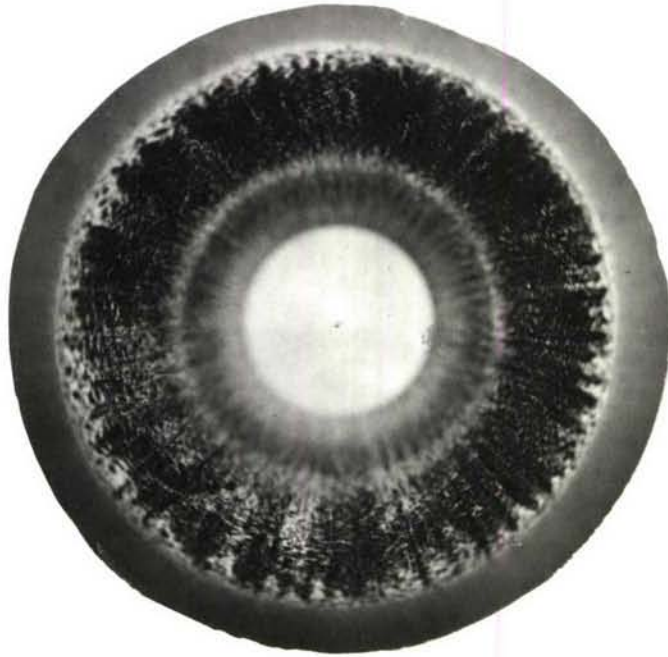
FIG.6. Barrel L/112. Ex M.E.L.F. Fired 1228 bombs obturated P.V.C. rings. Breech end view.
