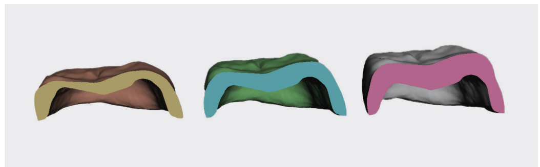
Figure 5: Cross sections of crown designs for 0.5mm, 1.0mm, and 1.5mm occlusal wall thickness.
