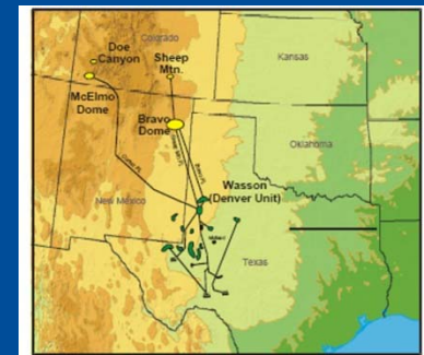
CO 2 flooding in the Permian Basin demonstrating CO 2 sources (yellow), flooded oil fields (green) and associated transmission lines.
