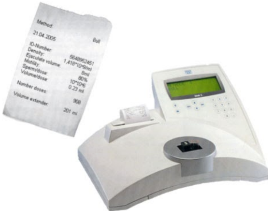
Figure 12. Photometer SDM5 for determination of sperm concentration, and automatic calculation of extender volume required and number of doses that can be produced from an ejaculate. (Courtesy of Minitube International).
