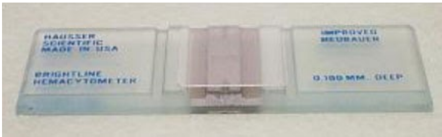
Figure 14. Hemacytometer with the Neubauer chamber. It requires an exclusively designed cover slip that comes in the original hemacytometer packaging. (Courtesy of the Melissa Rouge).
