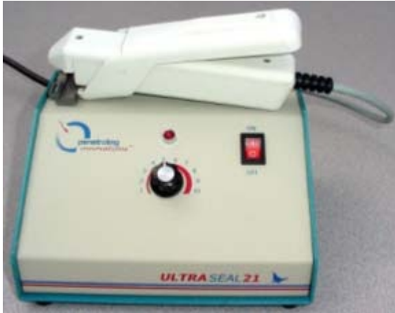
Figure 26. Ultra Seal 21, device that seals straws perfectly with ultrasound. No heat is produced at time of sealing. (Courtesy of Minitube International).
