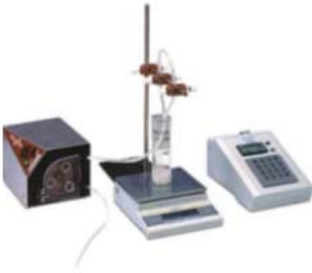
Figure 19. Smart dispenser to automatically and electronically add semen extender to an ejaculate. (Courtesy of Minitube International).
