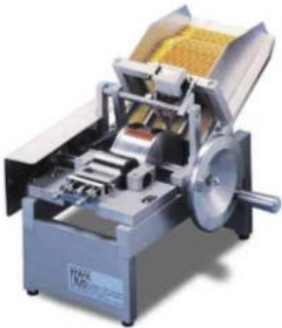
Figure 23. HDR manual straw printer for 0.5 and 0.25 ml straws. (Courtesy of Minitube International).
