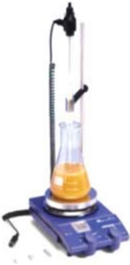
Figure 21. Magnetic stirrer with heater and contact thermometer. (Courtesy of Minitube International).
