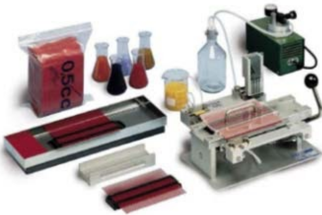
Figure 27. Semiautomatic Filling & Sealing Machine SFS 133 for both sizes of straws. Capacity: 2,000 straws/hour. (Courtesy of Minitube International).
