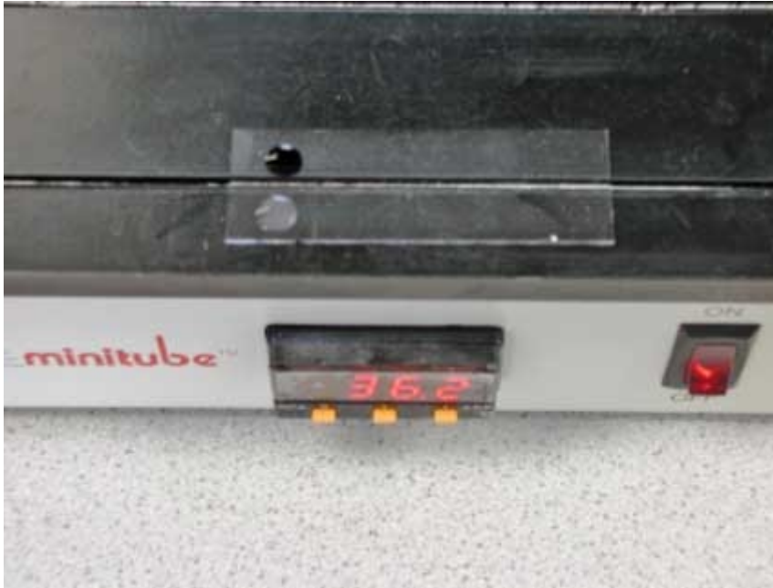
Figure 9. Glass slide on a warming plate with droplets of stain and semen before making a smear for sperm morphology evaluation.
