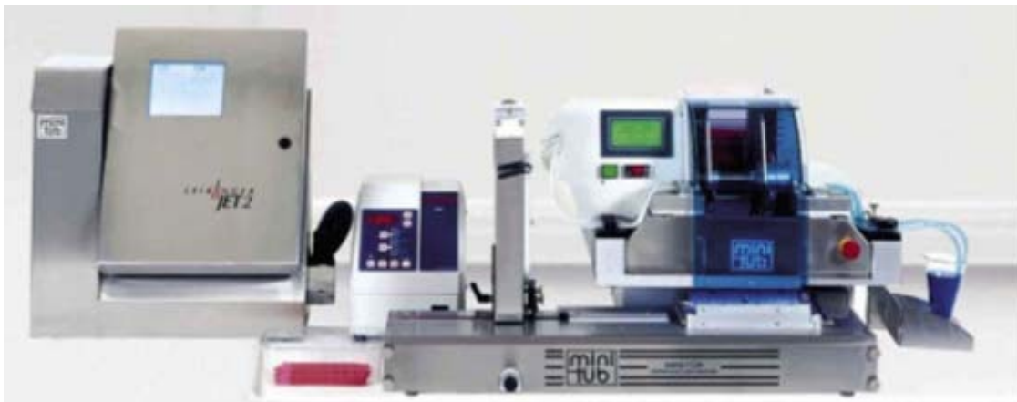
Figure 28. Mpp Quatro CombiSystem, automatic integration of straw printing, filling, and sealing in one step. Maximum capacity: 15,000 straws/hour. (Courtesy of Minitube International).
