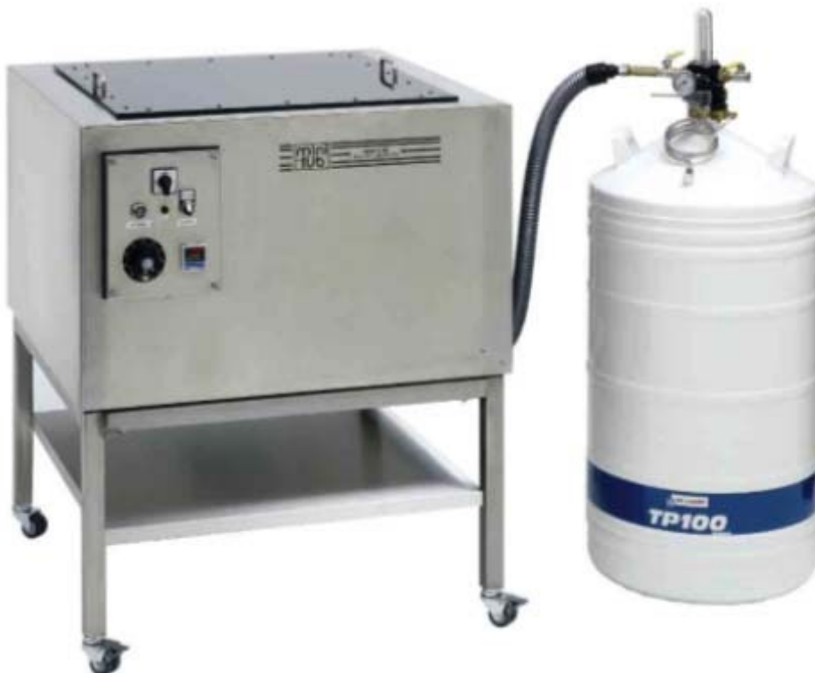
Figure 32. Semen Freezer MT with an automatic freezing curve from +5°C to -120°C with very low liquid nitrogen consumption. The dewar on the right has a capacity of 100 liters. (Courtesy of
