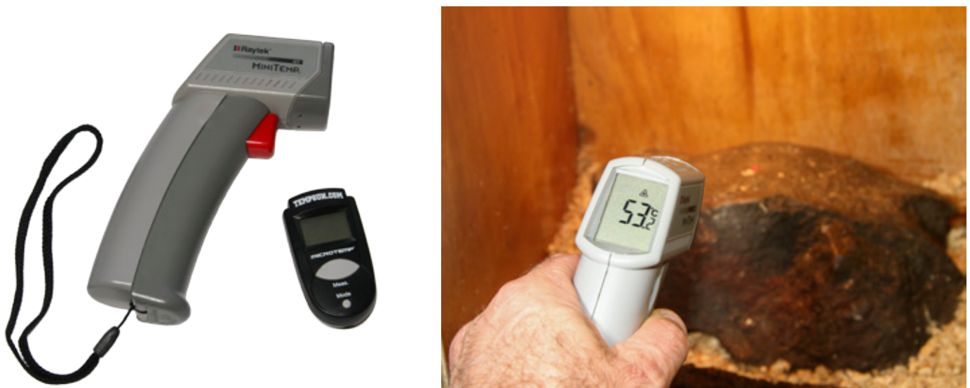
Fig. 2 Left: Infrared (IR) thermometers (non-contact temperature guns). Right: Measuring the basking temperature in an enclosure for hatchling lace monitors.
